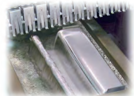
Turbulent wave for SMD and laminar wave for through-hole soldering
